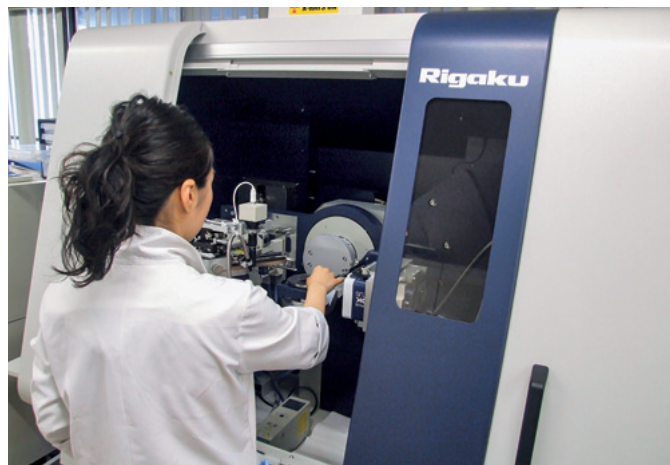
出土帯金具のX線回析分析 X-ray diffraction analysis of unearthed belt ornament
