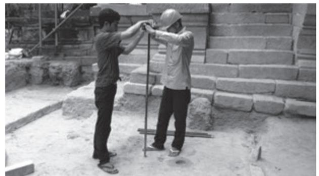
Fig. 4: Boring test using a hand auger
