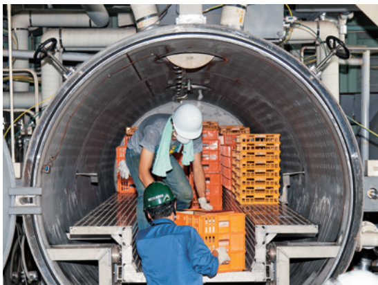
真空凍結乾燥機への搬入作業 Bringing the materials into the Vacuum Freeze Dryer
